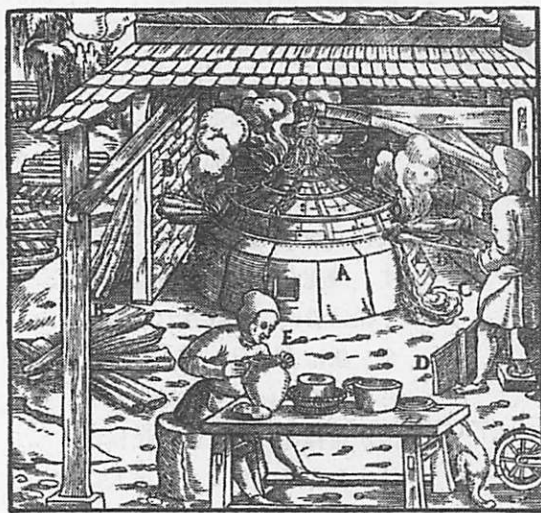
A—FURNACE. B—STICKS OF WOOD. C—LITHARGE. D—PLATE. E—THE FOREMAN WHEN HUNGRY EATS BUTTER, THAT THE POISON WHICH THE CRUCIBLE EXHALS MAY NOT HARM HIM, FOR THIS IS A SPECIAL REMEDY AGAINST THAT POISON.
